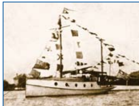
Oscar Nick’s first power boat, the yacht Kingfisher at anchor in full regalia. Note the shape of the hull and the substantial masts these early powerboats possessed due to the fact they could not rely on the early internal combustion engines and frequently had to revert to sail power to get back into port.
