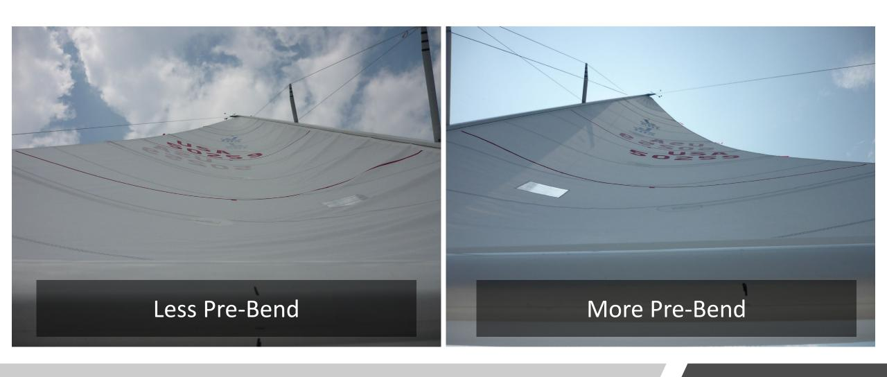
Basic Rig Tune- Pre-bend/Mast Bend
