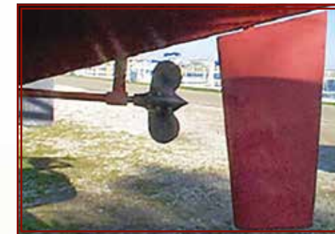
Both the rudder, and propeller & shaft have been painstakingly replaced for increased relative performance.
